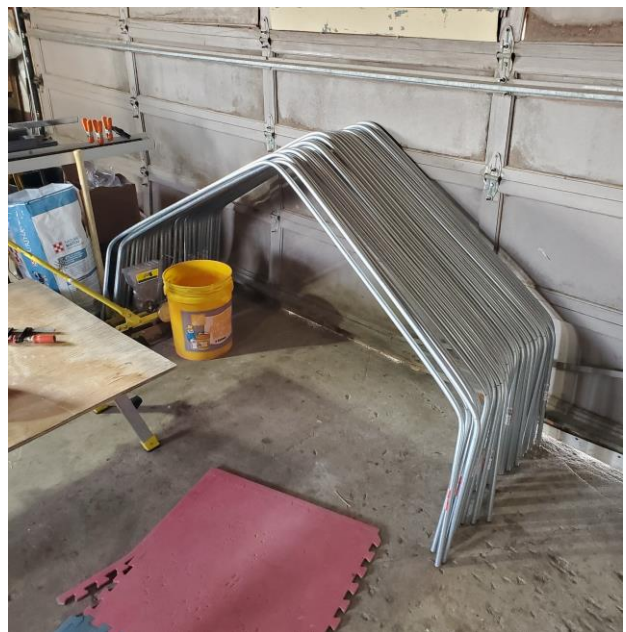
Photo of EMT bows. Bent on a simple jig made of wood and a pipe bender.
